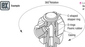
L-shaped Swivel plug is a product for the turn at the time of mold attachment. Because an 0 ring deteriorates when I face it about by die opening and shutting at the time of molding continually and causes an omission of water, please warm him.
